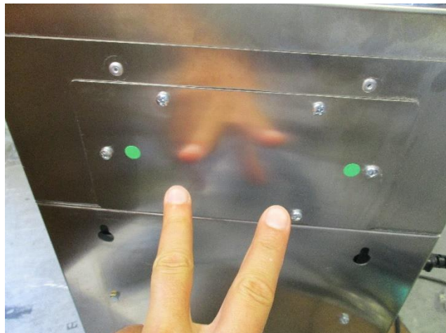
Electrostatic discharge immunity test: Points of application
