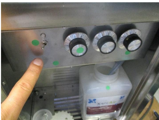
Electrostatic discharge immunity test: Points of application
