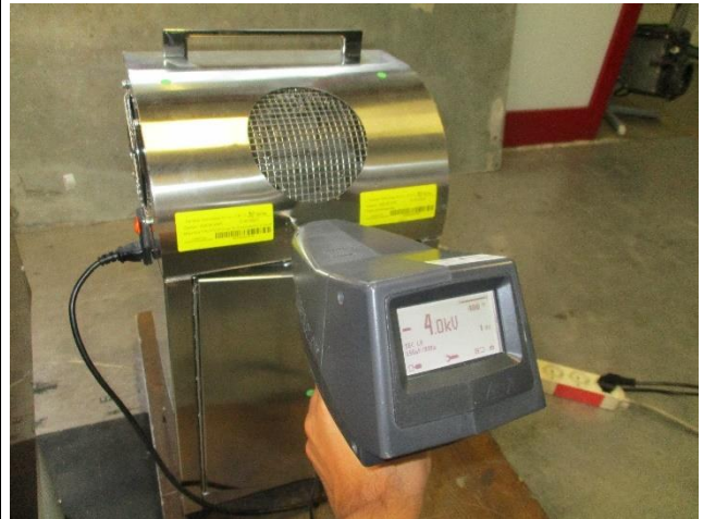
Electrostatic discharge immunity test: Points of application
