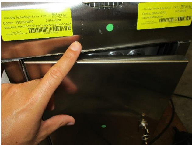
Electrostatic discharge immunity test: Points of application
