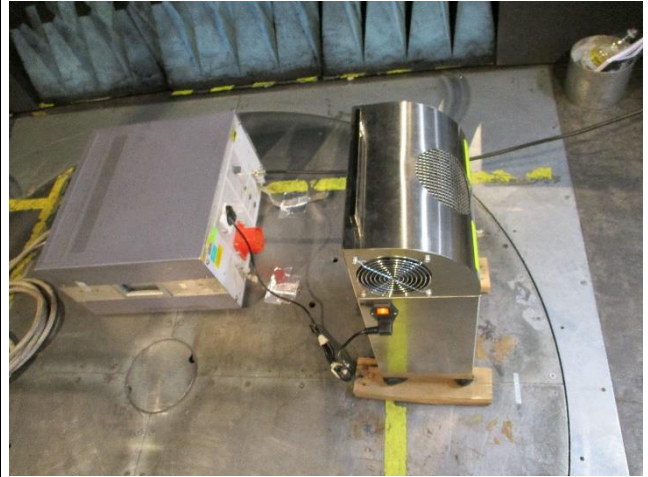
Measurement of disturbance voltage: cable's layout
