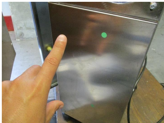
Electrostatic discharge immunity test: Points of application
