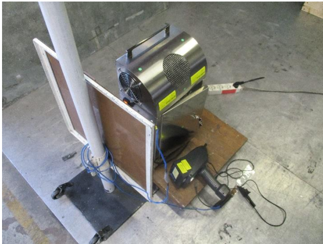
Electrostatic discharge immunity test: Points of application
