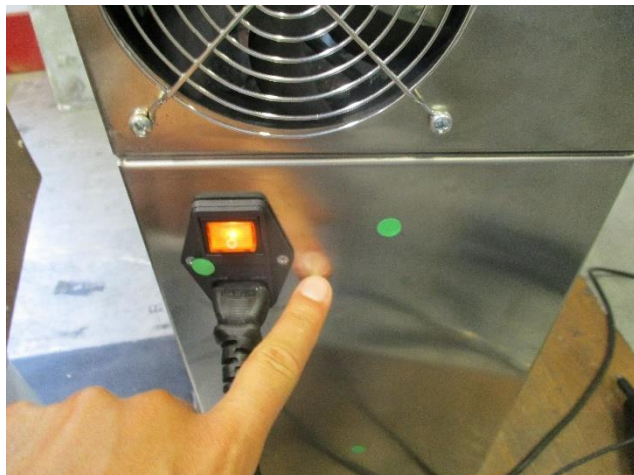
Electrostatic discharge immunity test: Points of application
